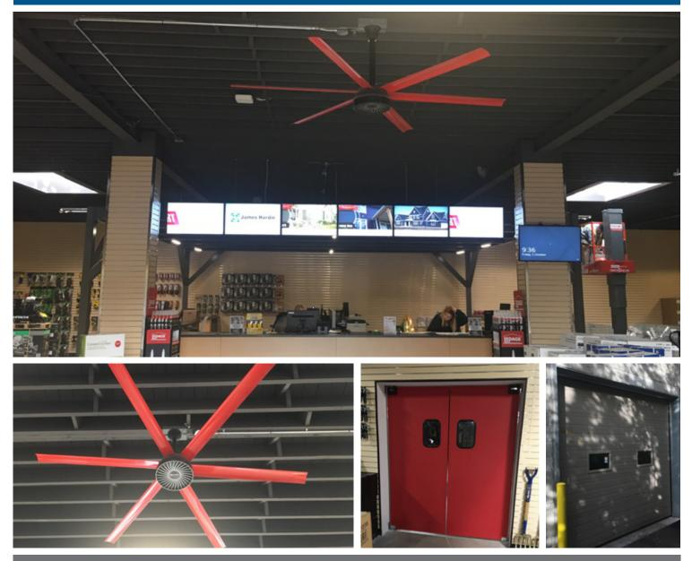
Address: 29 Connie Street, North York, ONArchitect: KingContractor: RiteStart LimitedCompleted: JuEquipment Provided:Garaga G-5000 Sectional Overhead Door & Liftmaster Model H Jackshaft OperatorEliason PE500 Impact DoorMacro Air AVD-370 8FT HVLS Fan
