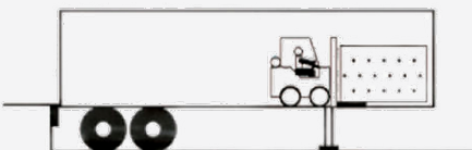
Unsupported trailer, completely dependent on landing gear
